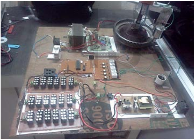
Fig. ceiling fan assembly, super capacitor bank, inverter, and microcontroller relay circuit.
